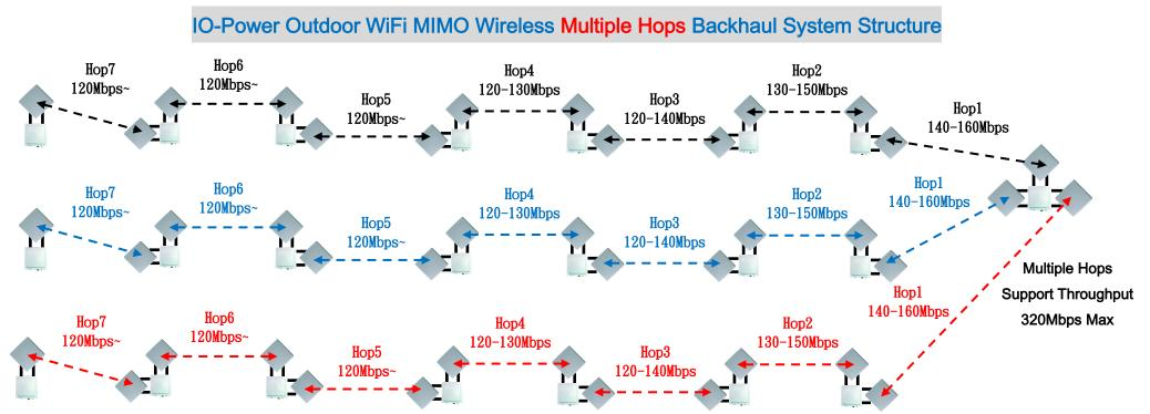
1. Design 2.4GHz & 5.8GHz dual band & 2\*2 MIMO Multi three RF modules backhaul system solution.
