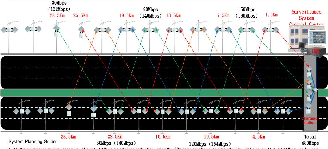
1. Multiple Hops each repeater hop, about 5~8Mbps bandwidth reduction, after the fifth repeater hops, the bandwidth will keep on 120~140Mbps, no longer reduces bandwidth.
