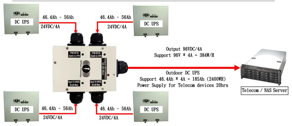
Insert 2 x 12~24VDC power supply voltage in series, the output voltage automatic step-up 24~48VDC power supply Insert 3 x 12~24VDC power supply voltage in series, the output voltage automatic step-up 36~72VDC power supply Insert 4 x 12~24VDC power supply voltage in series, the output voltage automatic step-up 48~96VDC power supply
