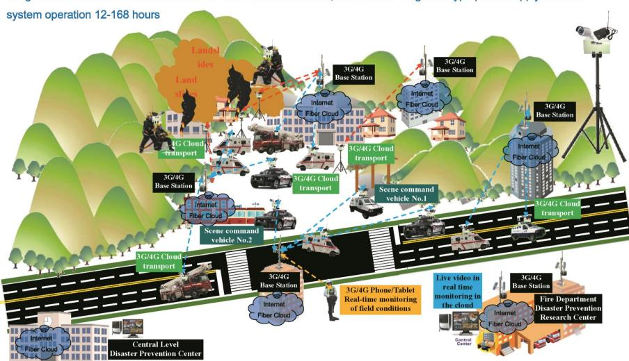
Emergency accident temporary \_ -3G/4G wireless mobile cloud surveillance system
