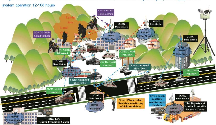
■ Construction site』 -3G/4G wireless video and real-time cloud network monitoring
