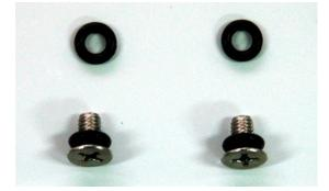
Then screw through another set of waterproof rubber gaskets, fixed on the stainless steel bracket
