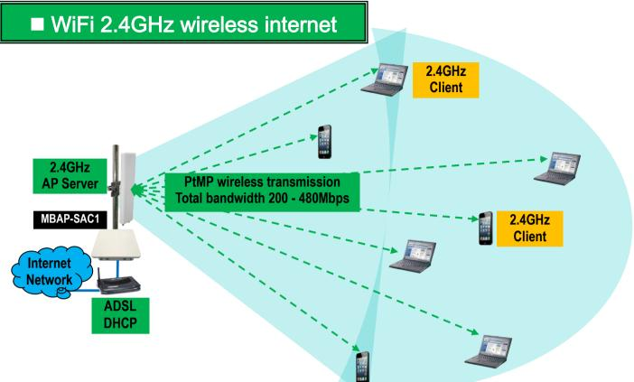
STA operation mode, which provides basic wireless client connection AP functions: STA (WDS) operation mode, acting as a PtP and PtMP client connection transmission application, through 802.11ac 2x2 MIMO wireless transmission technology, in the HT80 channel width setting, provide a single wireless network card module 867Mbps transmission rate and 480Mbps transmission traffic bandwidth, Suitable for monitoring image and data transmission backbone erection.
