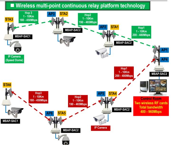
■ After the STA operation mode starts the high-speed mobile function, the mobile terminal STA supports the "automatically find the best transmission path function": (Auto Select Best Transmit Path Features)
