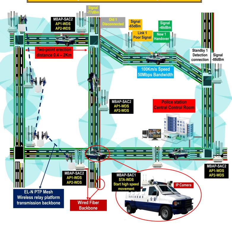
After the STA operating mode starts the high-speed mobile function, in order to solve the backup connection problem after the mobile client wireless connection is interrupted, the mobile STA supports the "Multiple fast automatic backup repair connection function": (Auto Multi-Fast Handover Backup Features)
