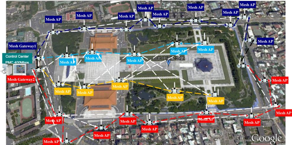
Outdoor WiFi wireless Mesh network backhaul redundant system with best path design descriptions
