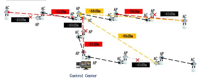
Every Wireless Station of wireless modules is running independently. According to the direction of transfer and scanning environmental by Site Survey. Then based on the scan results and set priority AP to connect. Due to failure or signal covered when connecting with AP, the Wireless Station will based on pre-set priorities for the AP's SSID and Cannel searching, communication, connection.
