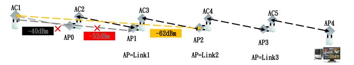
Recheck Time: 10 Min for AP1 (AP-Link1 Could not Link)
